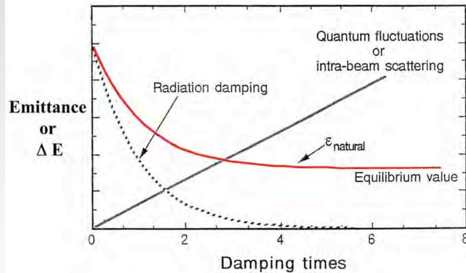
$$\begin{aligned}\varepsilon_{x,\min} &= 3.84 \times 10^{-13} \left( \frac{\gamma^2}{J_x} \right) F^{\min} \text{ meters} \\ &\approx 3.84 \times 10^{-13} \gamma^2 \left( \frac{\theta_{\text{achromat}}^3}{4\sqrt{15}} \right) \text{ meters}\end{aligned}$$
