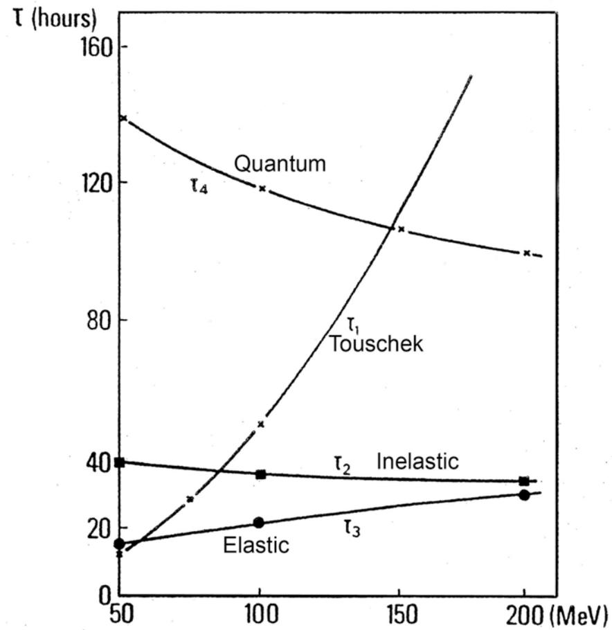
Fig. 1. Lifetime resulting from the different types of beam-gas interaction
